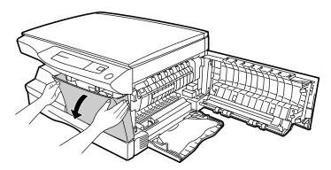
Remove the TD cartridge from the bag. Remove the protective paper. Hold the cartridge on both sides and shake it horizontally four or five times.
