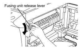
Gently remove the misfed paper from under the fusing unit as shown in the illustration. If the paper cannot be removed, proceed to "C Misfeed in the transport area".
