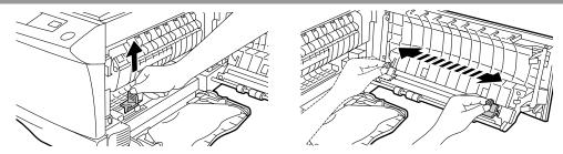
Return the charger cleaner to its original position. Close the side cover by pressing the round projections near the side cover open button.
