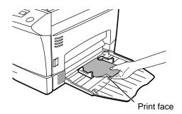
Press the tray select () key to select the bypass tray. Set the number of copies if using standard copy paper. Press the print () key.
