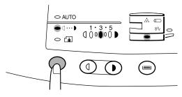
Use the light (①) and dark () keys to adjust the exposure level. If exposure level 2 is selected, the two left-handmost indicators for that level will light up simultaneously. Also, if level 4 is selected, the two right-handmost indicators for that level will light up simultaneously.
