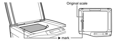
Gently close the original cover. When copying a book or an original which has been folded or a crumpled original, press down the original cover lightly. If the original cover is not securely closed, the copies may be striped or blurred.
