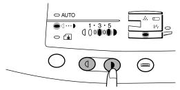
Set the number of copies using the copy quantity  $( \^{} )$ ,  $( \^{} )$  keys and press the print  $( \^{} )$  key.
