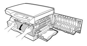
**2** Gently pull the TD cartridge out while pressing the lock release button. Dispose of the old TD cartridge in accordance with local regulations.
