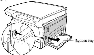
Remove the CAUTION tape from the front cover and remove the two protective pins from the fusing unit by pulling the strings upward one at a time.
