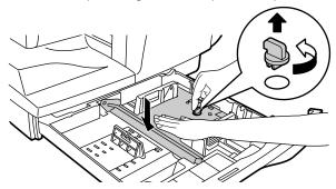
Store the pressure plate lock which has been removed in step 2 and the screw which has been removed when unpacking (see page 11, step 2 of **REMOVING PROTECTIVE PACKING MATERIALS**) in the front of the paper tray. To store the pressure plate lock, rotate the lock to fix it on the relevant location.
