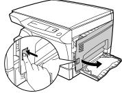
**2** Check the misfeed location. Remove the misfed paper following the instructions for each location in the illustration below.
